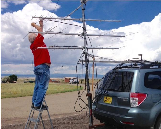
My rover, configured for 50MHz to 2304 MHz is shown above. There is a 24 GHz Gunnplexer in the car. The TS-2000X covers 50, 144, 432 and 1296 Mhz. I use 222 Mhz and 902 Mhz transverters to activate the additional bands. Most contacts are made on SSB or CW but I'm working more contacts lately on FM as well, and they really help. The picture above was taken during the June 2015 VHF/UHF contest in DM74, near the Tarrant County landfill; a favorite operating spot near the Moriarty grid convergence.
